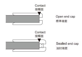
If the end cap is not securely installed to the outer casing, the outer casing might not operate properly.
