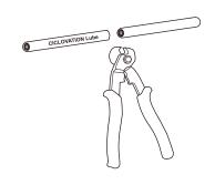
3. After cutting, use the cable cutter to correct the distortion of the outer casing. And install end caps.
